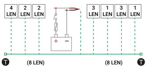
Note: Do not connect the NMEA 2000® power cable to the same terminals as the engine start batteries, autopilot computer, bow thruster or other high-current devices.
